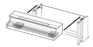
At this time the screws on the bottom of the piano (3) should hook into the cutouts in the stand brackets (9).
