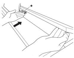
The support bracket is designed to prevent sudden closing of the lid. Should the support bracket stop moving, once again press back on it (\*) as you slowly and carefully lower the lid.
