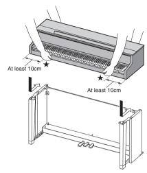
Place the piano onto the stand starting the Digital
