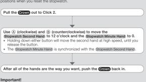
Timekeeping stops while the crown is pulled out. Correct the current time setting after performing the above operation.
