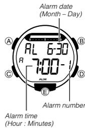
You can set up to three independent multi-function alarms with hour, minutes, month, and day. When an alarm is turned on, the alarm tone sounds when the alarm time is reached. One of the alarms has a snooze feature. You also can turn on an Hourly Time Signal that causes the watch to beep twice every hour on the hour.
